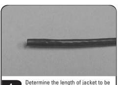
removed from the twisted-pair cable. Using the Siemon Cable Preparation Tool with the yellow die, proceed to step 2
