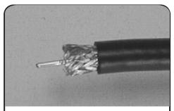
Remove the cable from the preparation tool and remove the scored sections of the cable jacket exposing the grounding braid and center conductor.
