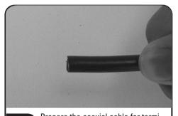
Prepare the coaxial cable for termination by squarely cutting the end of the cable. Using the Siemon Cable Preparation Tool with the black die, proceed to step 2.
