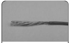
Remove the cable from the preparation tool and remove the scored section of cable jacket.
