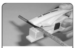
Squeeze the tension arm of the preparation tool and insert the cable to the desired length. Hold the cable close to the tool body and rotate the tool around the cable.
