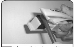
Squeeze the tension arm of the preparation tool and insert the cable until the end of the cable contacts the stop. Hold the cable close to the tool body and rotate the tool around the cable three times.
